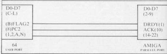
Cable Wiring For Parallel Data Transfer
